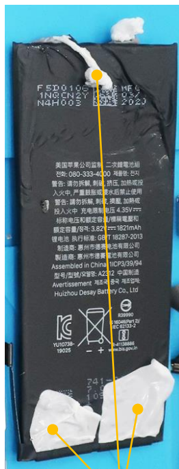
Battery placement by double-sided tape
